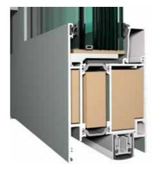
The CS 77-FP EI3O and EI6O is developed based on the existing CS 77 profiles and accessories for windows and doors and extensively tested in an optimized European test and approval program. The fireproofing time span is achieved by inducing a special cooling material into the profile chambers and by using self-adhesive and water-resistant swelling gaskets. These gaskets do not need to be sealed, reducing fabrication time of the profiles and saving costs.
